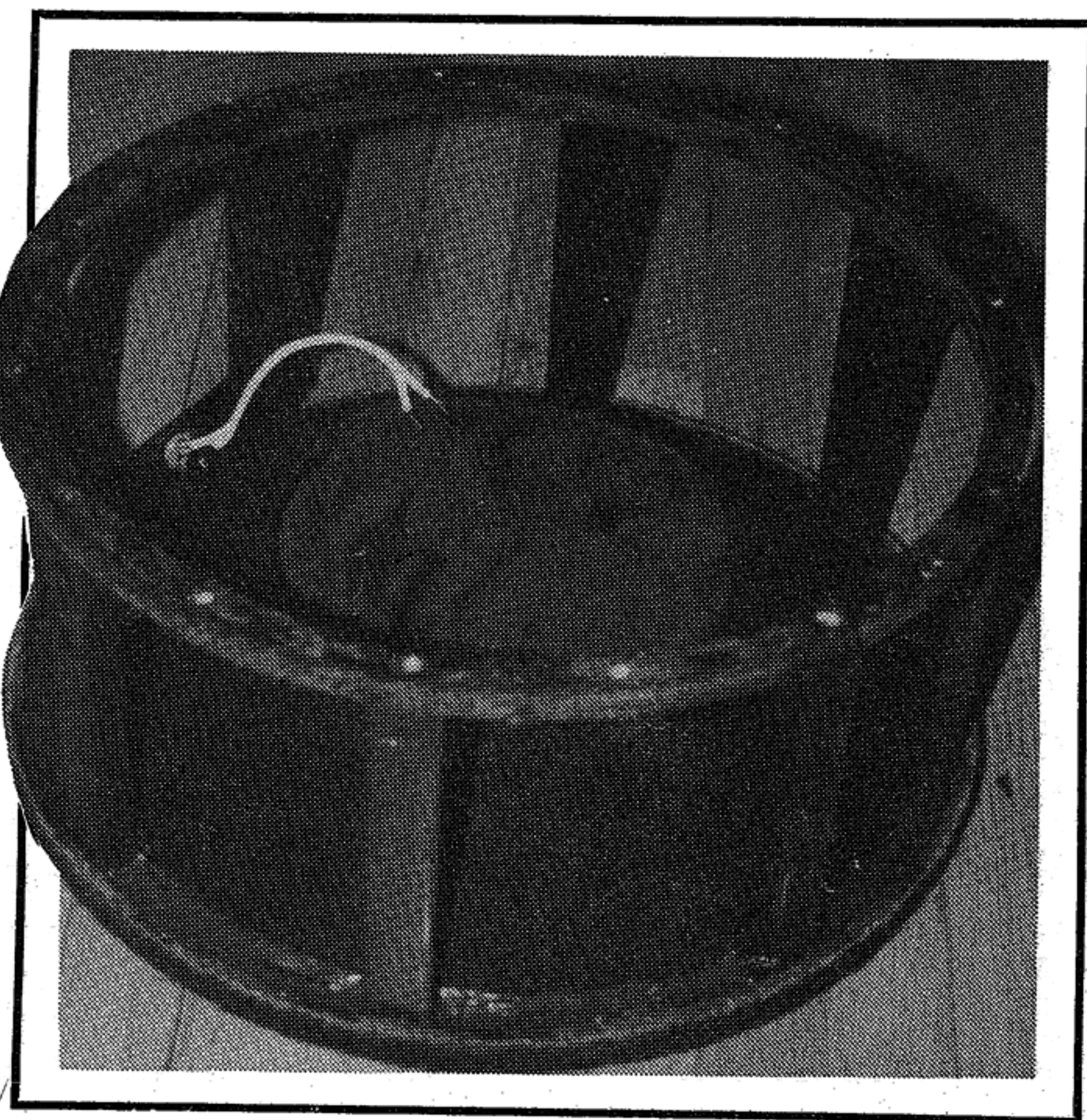
PHOTO 9: A completed revised speaker basket with the reflecting cone epoxied in place. The interior of the cone is stuffed with wool, and black grille cloth holds the wool inside the cone. Note the input jack and wire terminations for attachment to the woofer.
