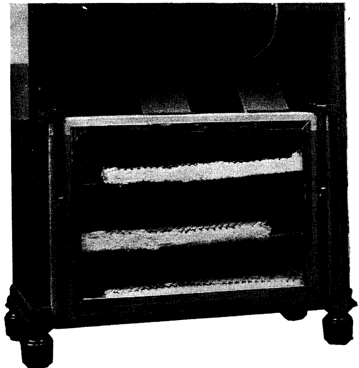
Acoustical labyrinth with back removed
