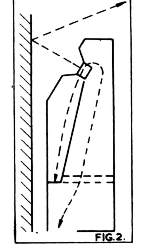
frequencies from a suitable height. A length of approximately 5 feet gives a nominal column resonance of just under 50 c/s. The unit is tilted slightly to allow most of the reflected sound to clear the cabinet top.
