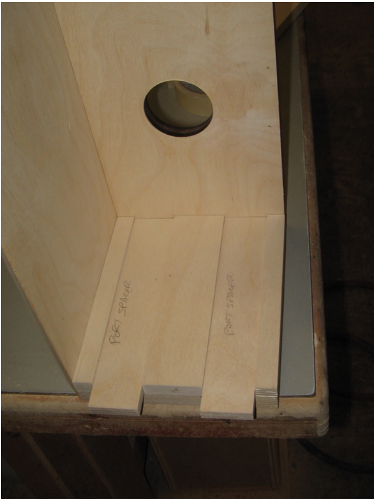
Three port divider blocks – use provided spacers
